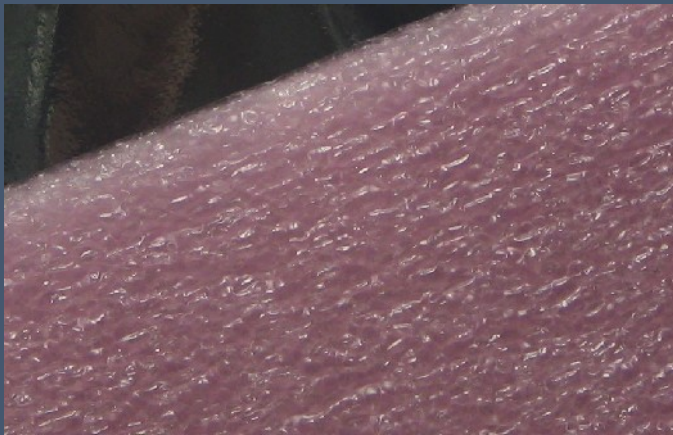
Pink Antistatic Polyethylene Foam
